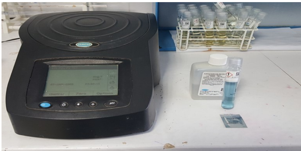
Figure 22 : dosage de nitrite (NO 2 - )
