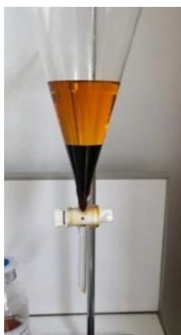
Figure 2.4 Crude biodiesel and glycerol layers.
