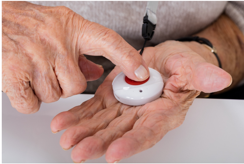
Figure IV.7: Example of an intelligent device for tele-assistance of aged and sick persons. Source [11].
