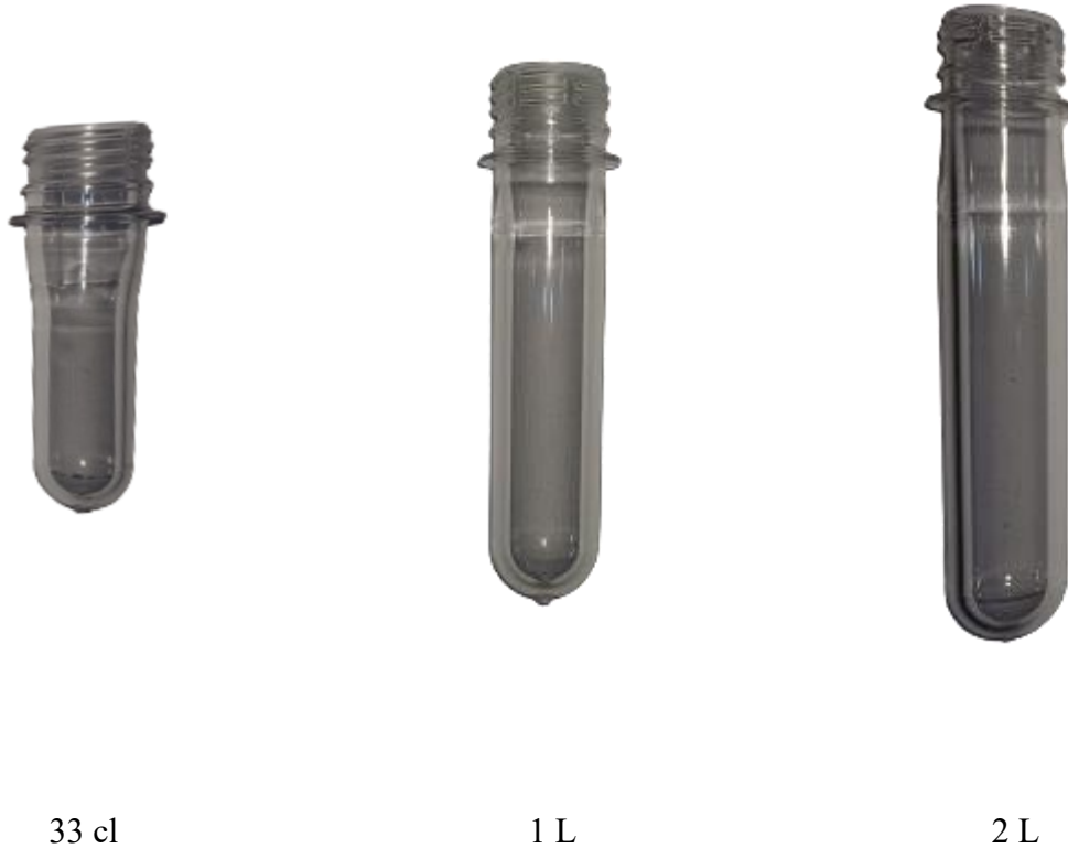
Fig 8. Variation in PET Bottles Preforms
