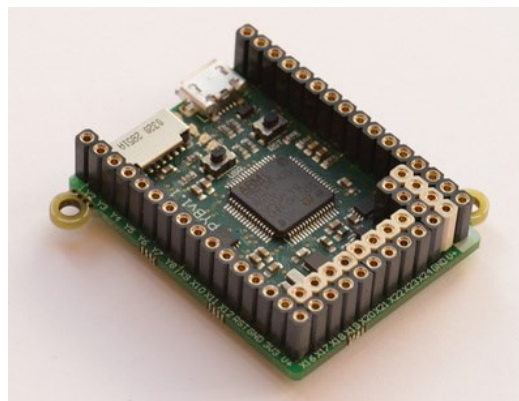
Figure 44. Example of a MicroPython microcontroller board (the pyboard) [153](STM32F405RG microcontroller, 168 MHz Cortex M4 CPU, 1048KB flash ROM and 196KB RAM)
