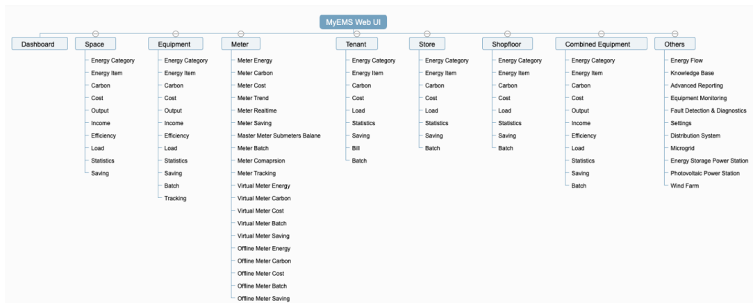
FIG. 5.4: Module-based navigation structure of the MyEMS system.
