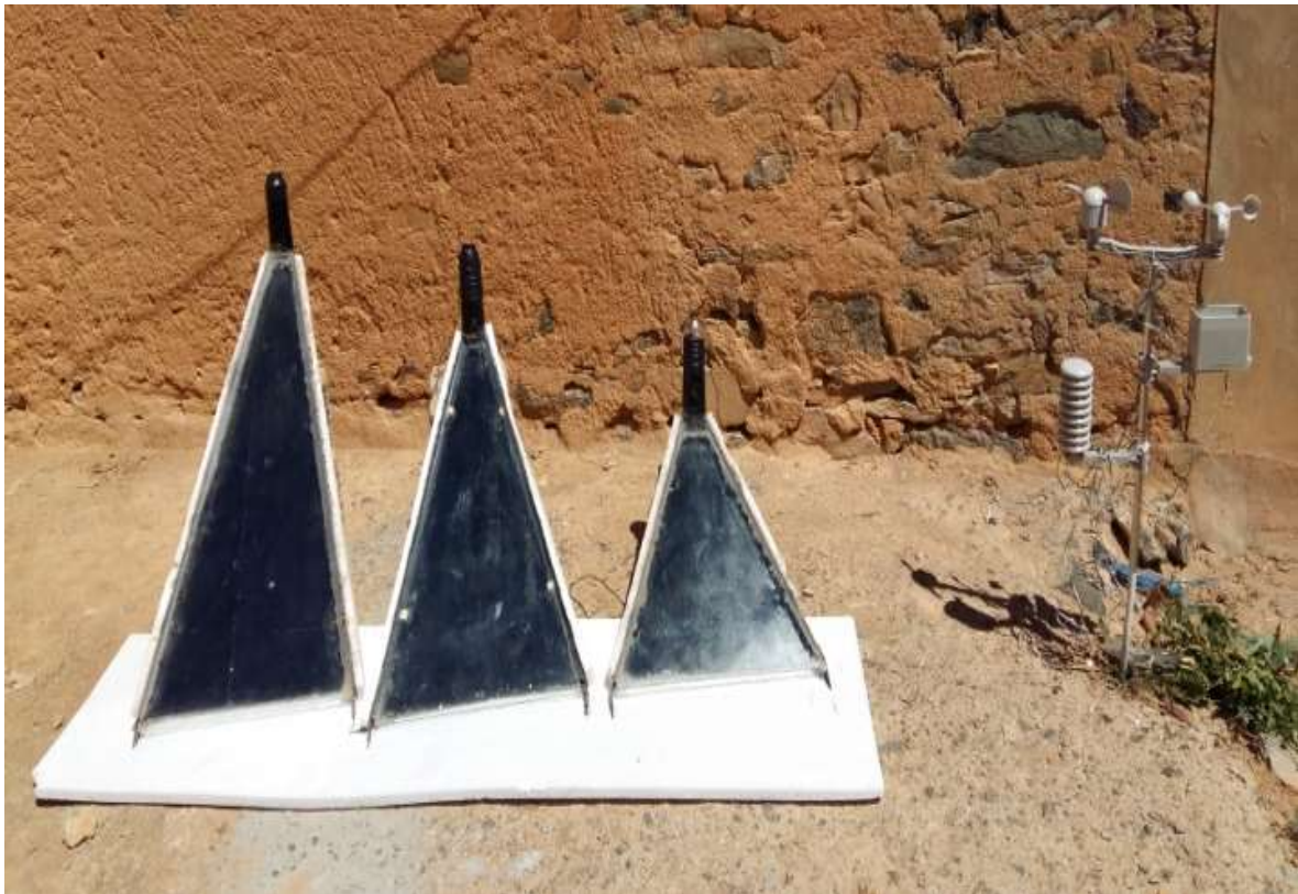
Figure II.2: Solar chimneys and weather station installation
