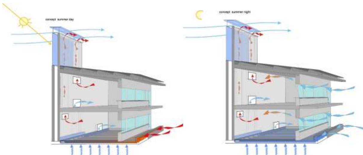
Figure I.24: Ventilation and traditional cooling techniques in a school in Damascus [45]
