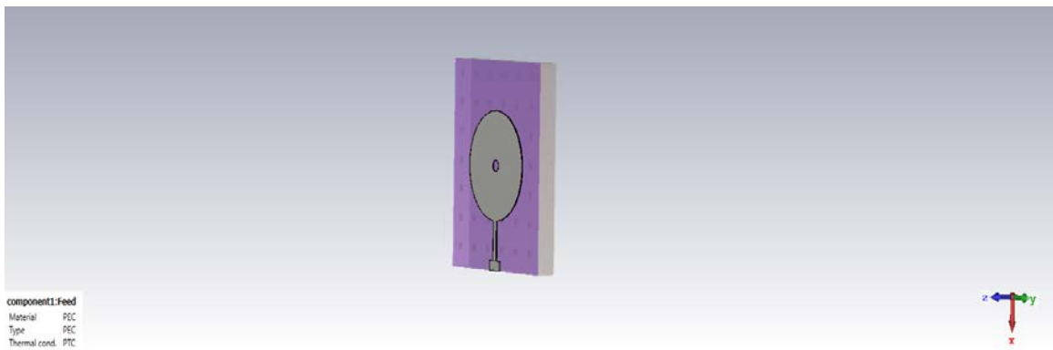
Figure III- 6. Structure d'antenne patch.
