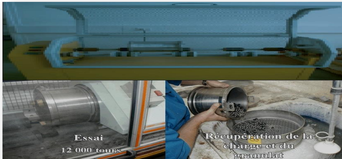
Figure 3. 8: Essai Micro Deval.
