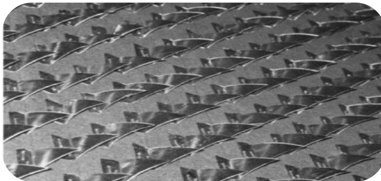
Figure II.7 : Disposition des obstacles DCL.
