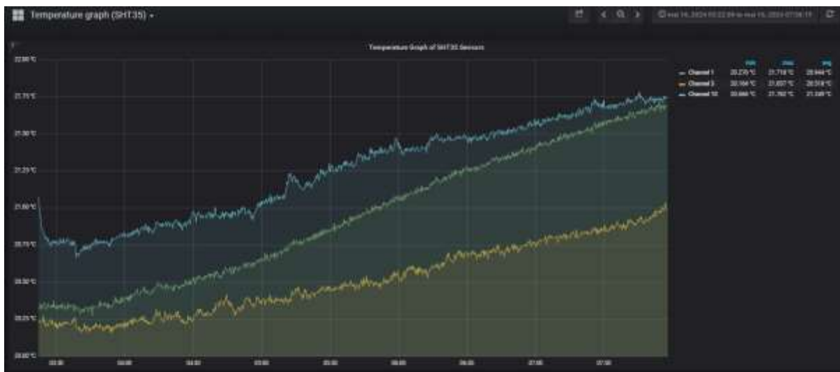
Figure III-11 Temperature Graph of SHT35 Sensor
