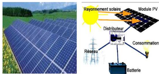
Figure (I.3) Système photovoltaïque [1]
