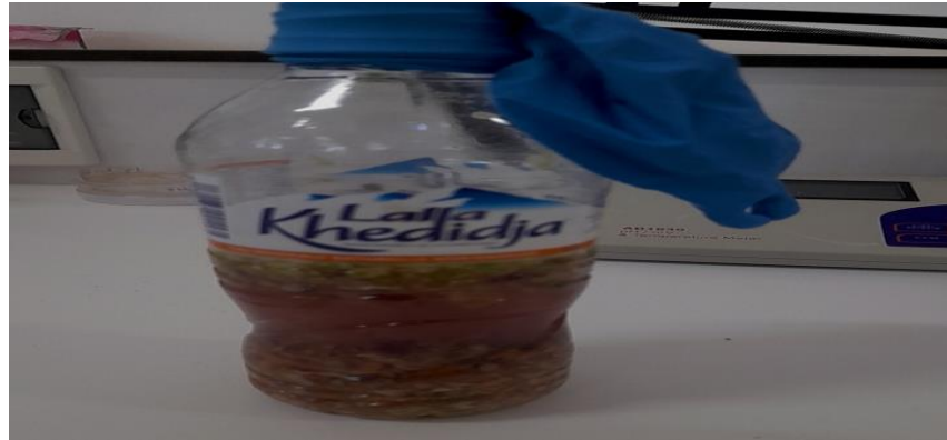
Figure IV-5 Simplified Methanization Test
