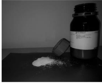
Fig.1.28. Photograph of Al 2 O 3 nanoparticle powder prior to addition
