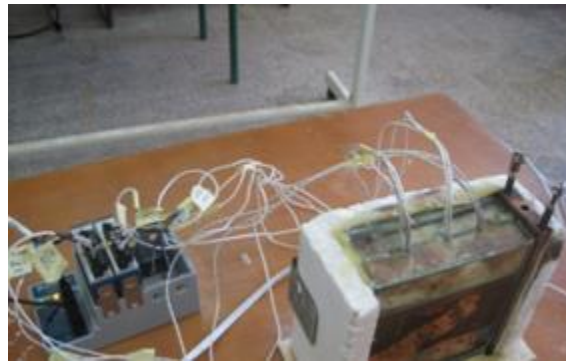
Fig. 3.6. Connection of thermocouples to the NI acquisition chain
