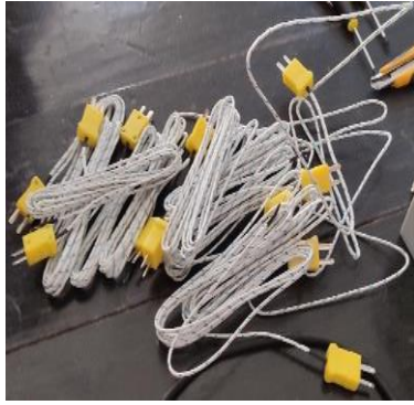
Fig. 3.18. Type K sensors with flat heads used in experiments
