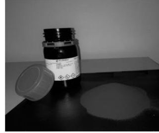
Fig.1.29. Photograph of Cu nanoparticle powder prior to addition to PCM.
