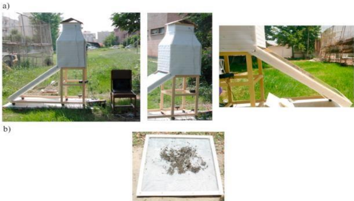
Figure I.17: (a) Photos of the tested solar dryer, (b) Final dried product from each trial.
