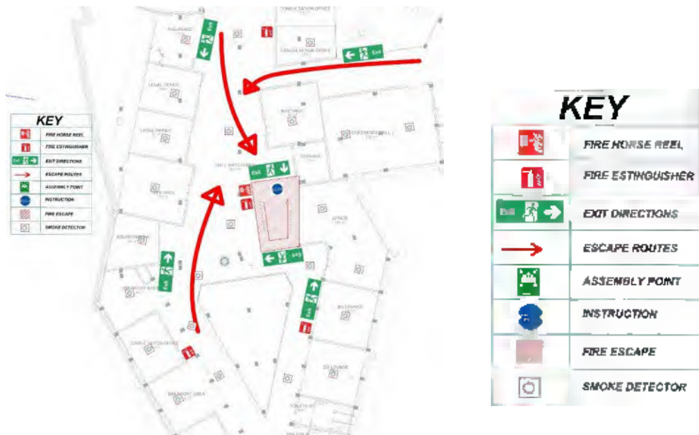
Figure 136: First Floor Fire Escape Plan: Source (Author)
