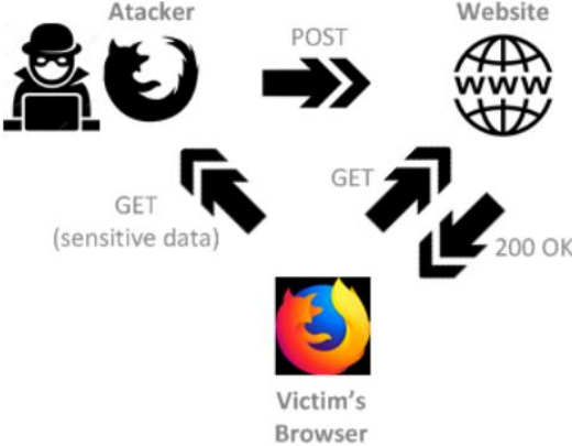
Figure 5: Scenario for a reflected or indirect XSS attack
