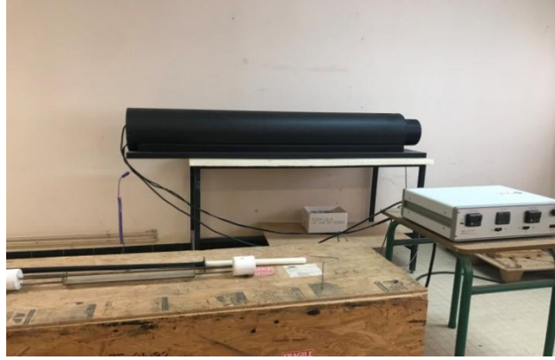
Fig. 17- Demagnetization using an oven.
