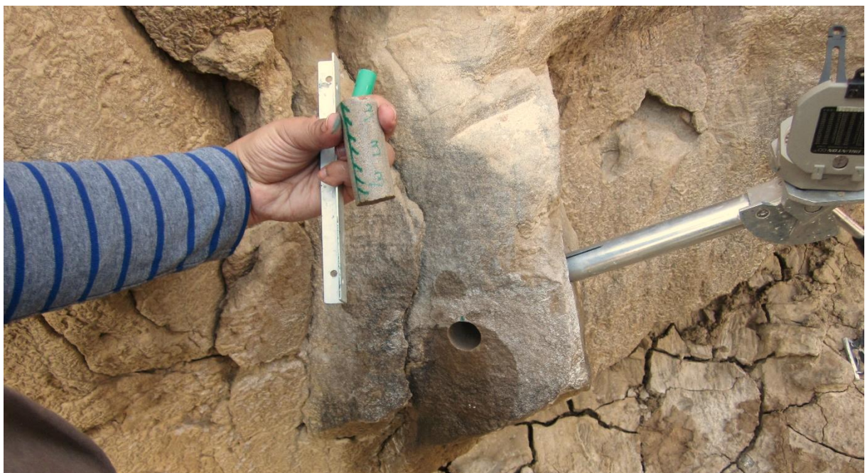
Fig.11- Sampling method using a core driller.
