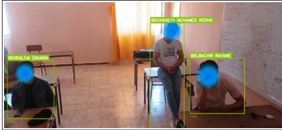
FIGURE 3.16: Classroom recognition test using YOLOv8-Face detection and InsightFace (ArcFace) recognition.
