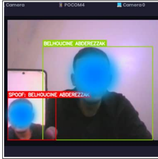
FIGURE 3.8: Anti-spoofing test. The real live face is accepted, while the presentation attack displayed on a phone screen is marked as SPOOF .
