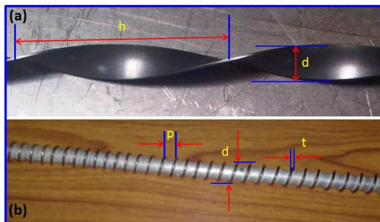
Figure II. 10 Images des inserts (a) ruban torsadé (b) bobine de fil [24]
