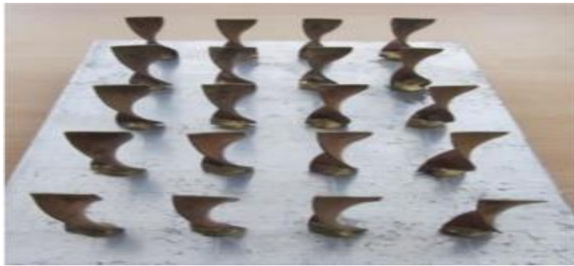
Figure II. 25 Arrangement de bandes torsadées [52]
