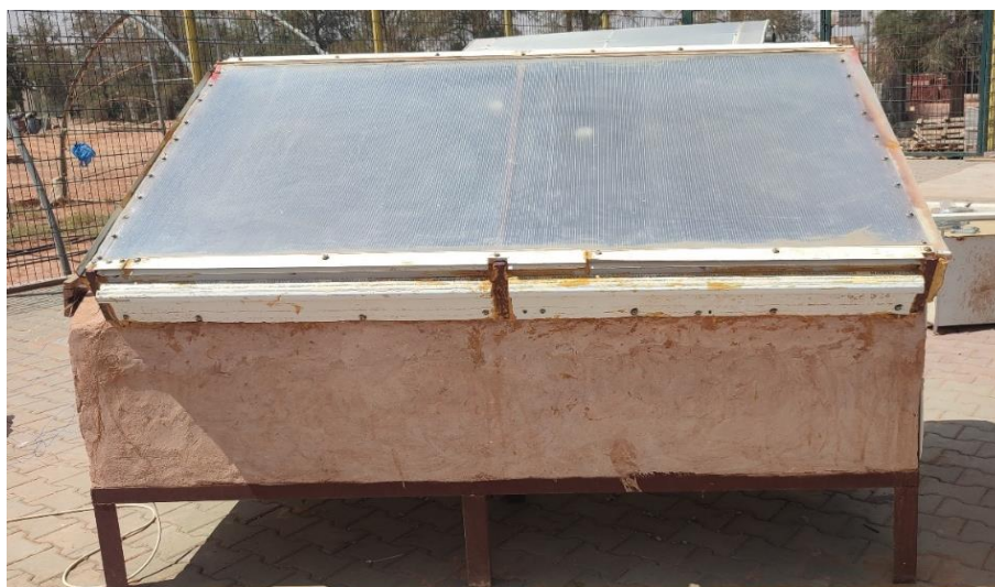
Figure II. 3. Image and illustration of the clay based direct solar dryer
