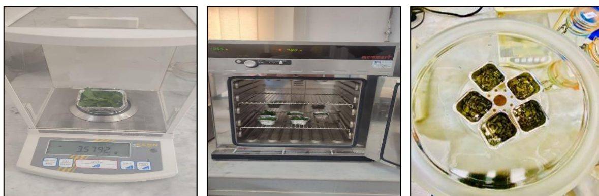
Figure II. 7. Moisture content determination process
