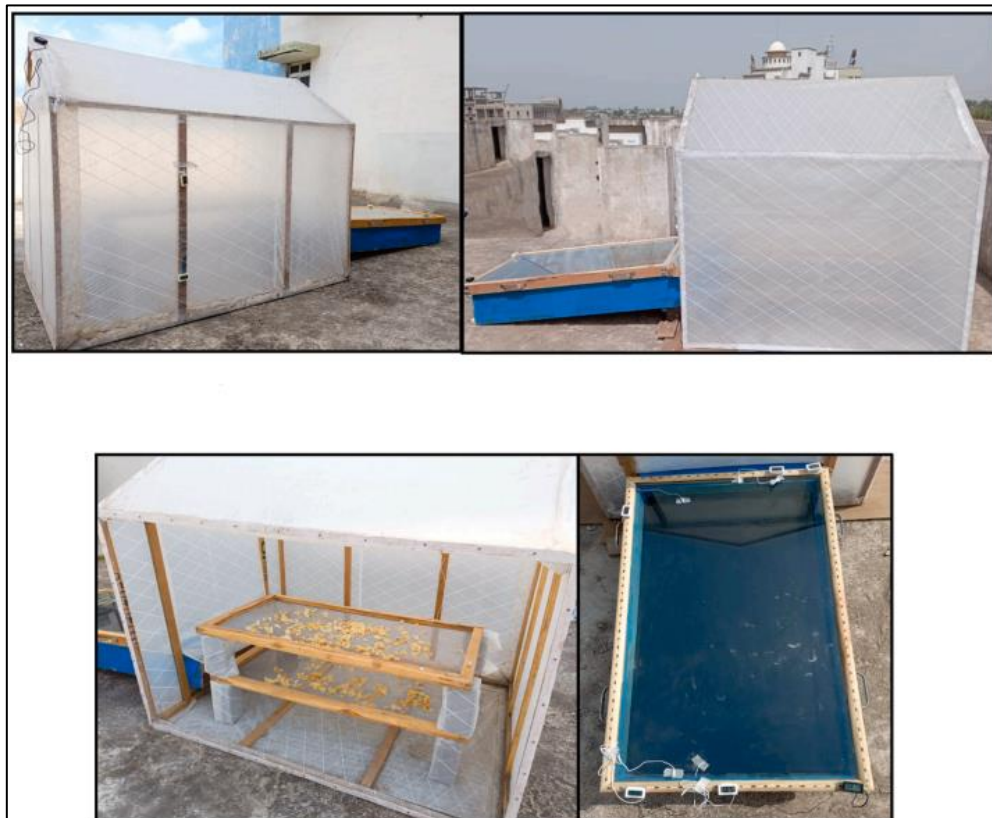
Figure I. 16. Tent house solar dryer [62]
