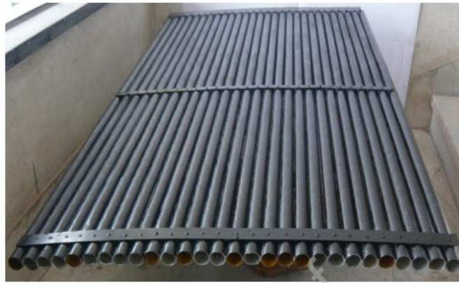
Figure II.9: The absorber of the TSAH
