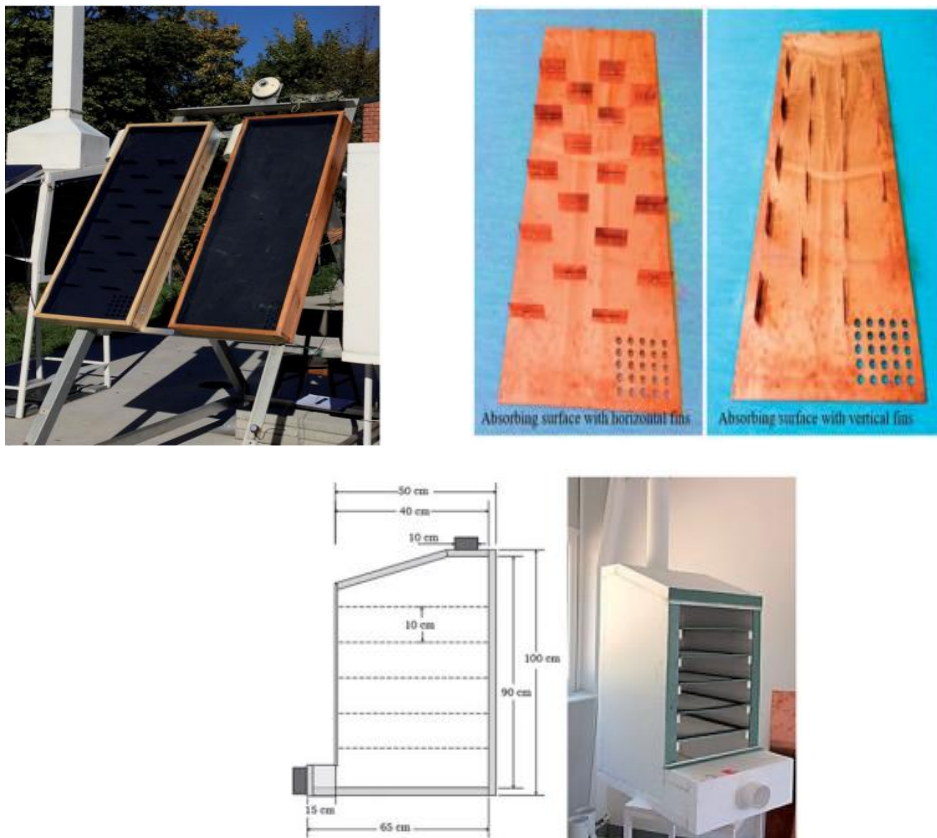
Figure II.5: (a) installation of solar drying system (b) Directions of fins on the absorbing surfaces of collectors (c) Design of drying chamber
