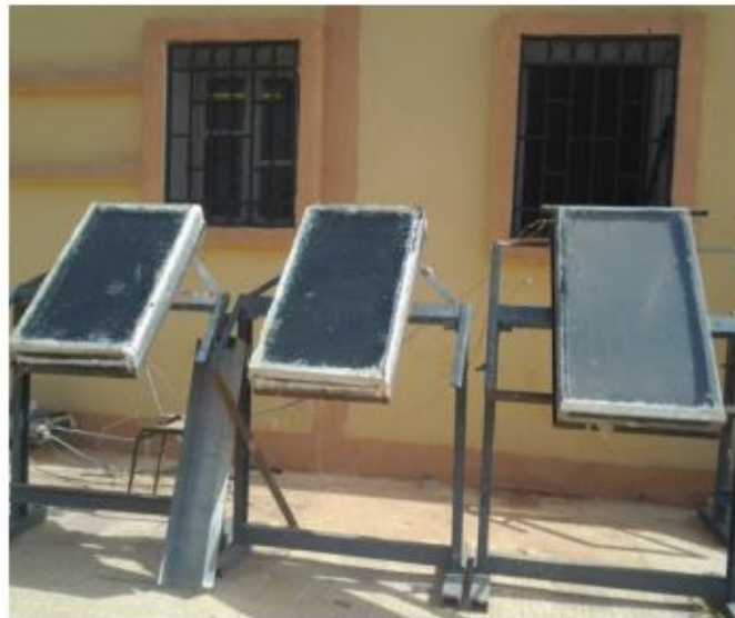
Figure II.12: Photo of the solar air collector
