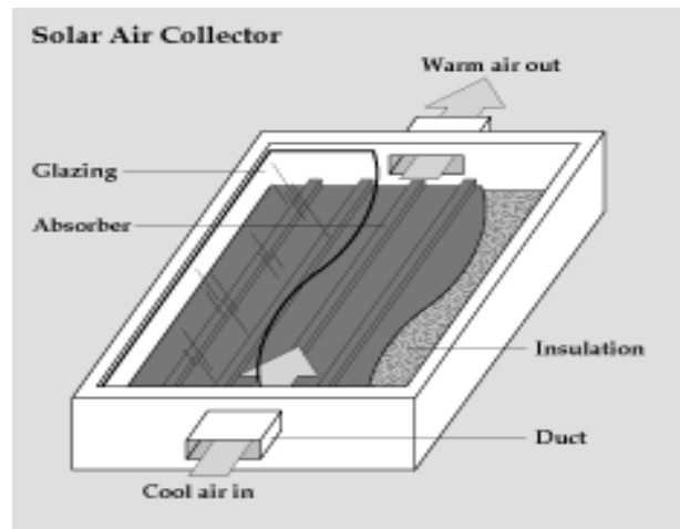
Figure I.4:Flat based air solar collector
