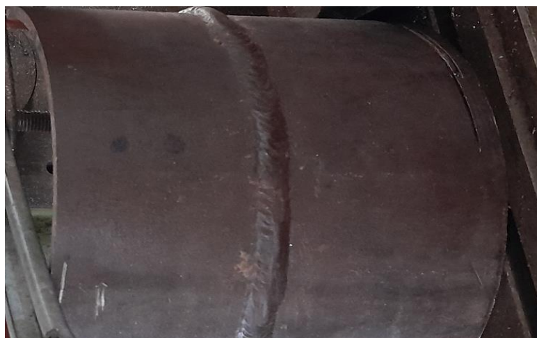
Figure 2. 1: Morceau de pipeline soudé
