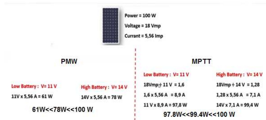
Figure 1 27 Difference between the controller PMW and MPPT
