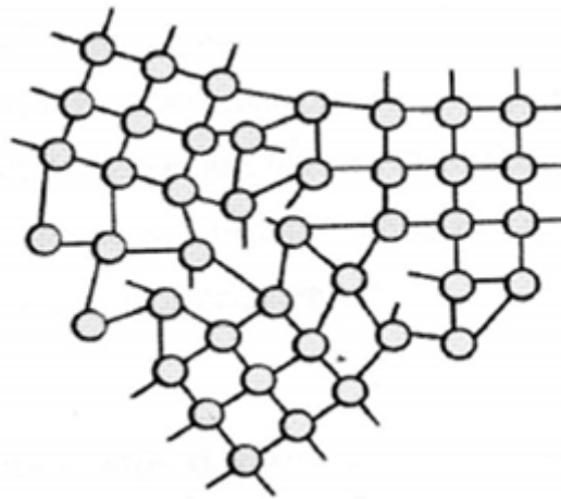
Figure 1 6 Microcrystalline silicon atomic structure [20]
