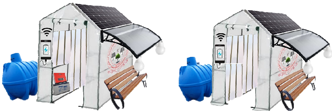
Figure 3 16 Schematic of Sustainable Disinfection Tunnel (SDT)[76]
