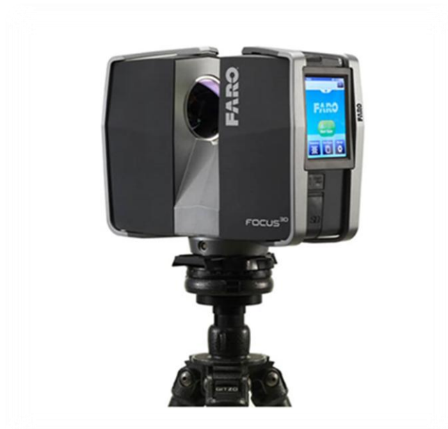
Figure 12 : Scanner laser terrestre FARO FOCUS 3D X130
