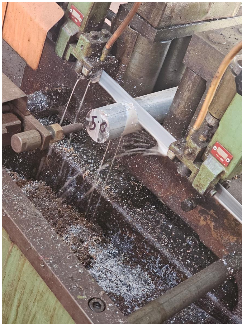
Fig III.6: Cutting the aluminium alloy workpiece on a band saw
