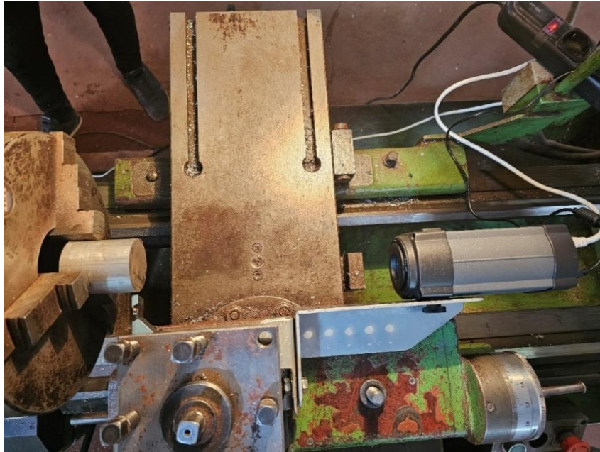
Fig III.12: Camera mounted in front of the cutting tool.
