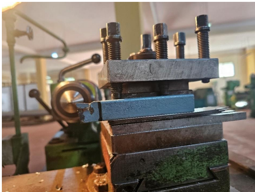
Fig III.11: Aligning the tool with the centre.
