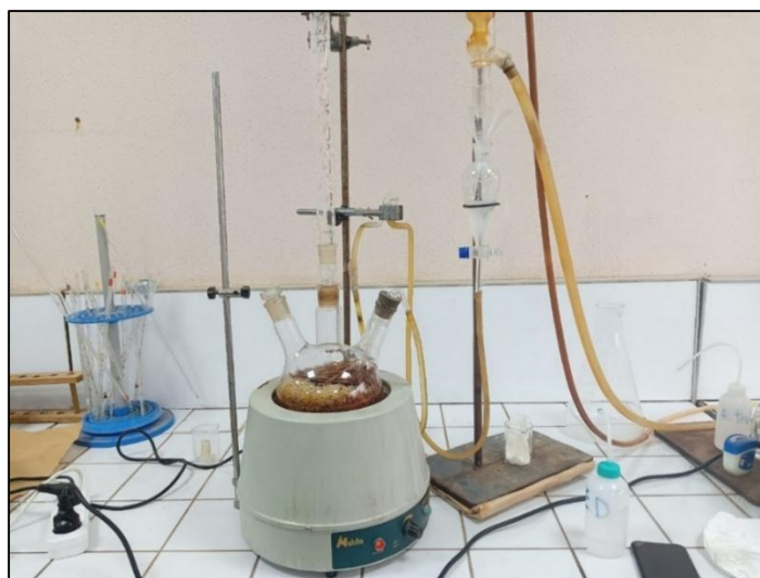
Figure 6: Hydrodistillation apparatus for the extraction of Cinnamomum verum essential oil
