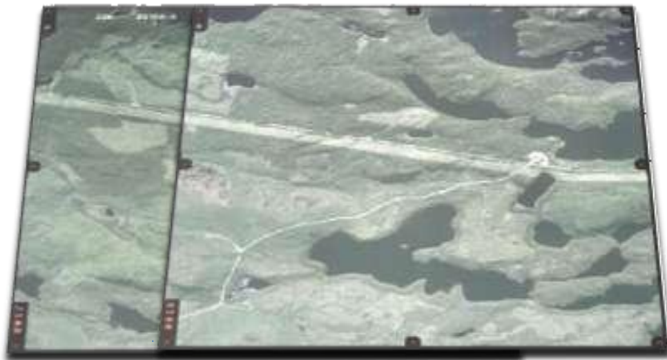
Figure 13. Zone de recouvrement longitudinale Source CCRS/CCT
