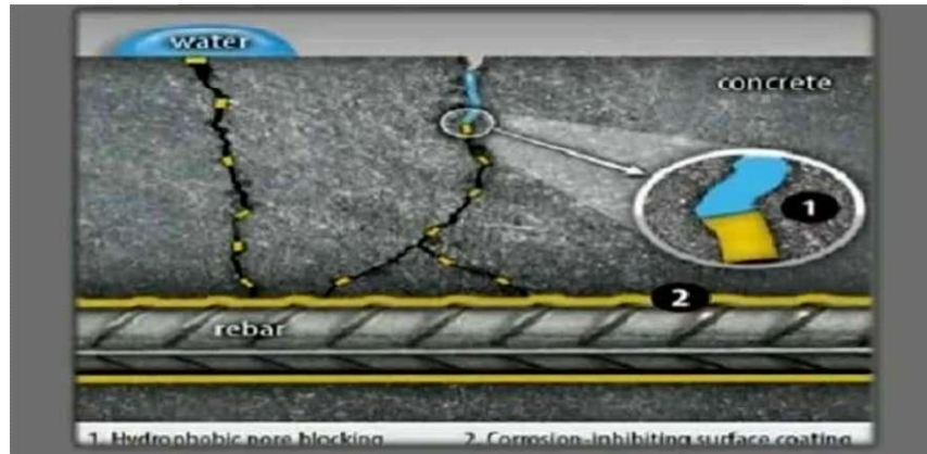
Figure I.9: Concrete permeability mechanism [43].
