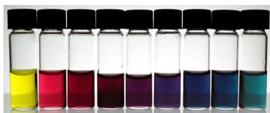
Figure 1.6 : Effect of gold nanoparticle size on the apparent color of colloidal solutions [19].
