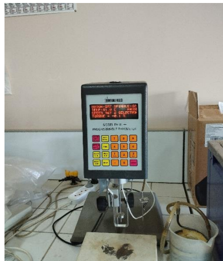
Figure II. 9: Rhéomètre programmable Brookfield MODEL DV -III+
