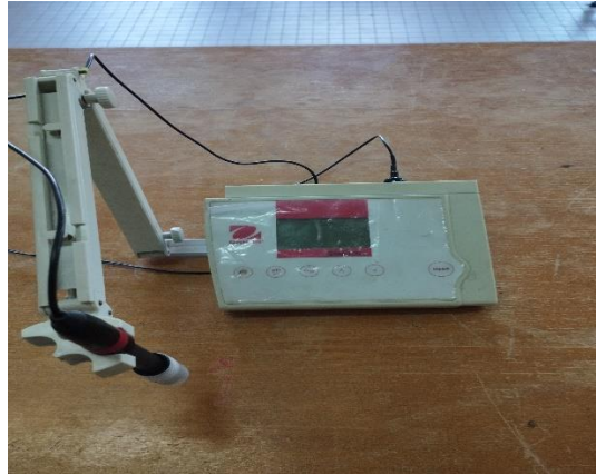
Figure II. 5: pH-mètre Ohaus -Starter 2C, Electrode Ohaus -SC210
