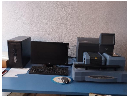
Figure II. 7 : Appareil TA-Q600 couplé DSC/ATG
