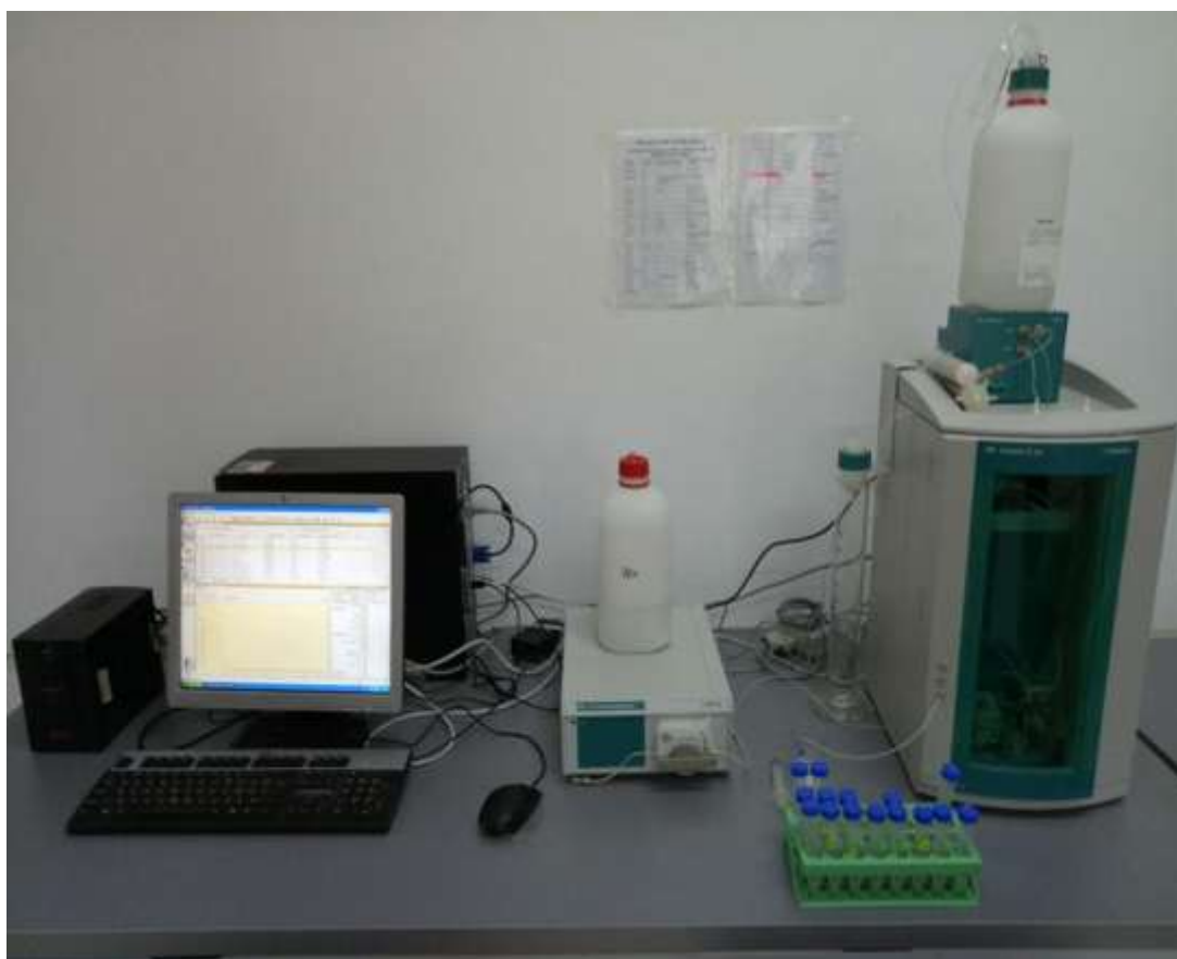
Figure II.1 : chromatographie ionique model (881 Compact IC pro )
