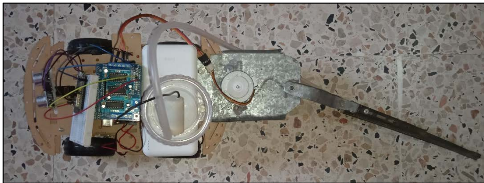
Figure III.23 Overhead view for prototype of the disinfection robot during integration test
