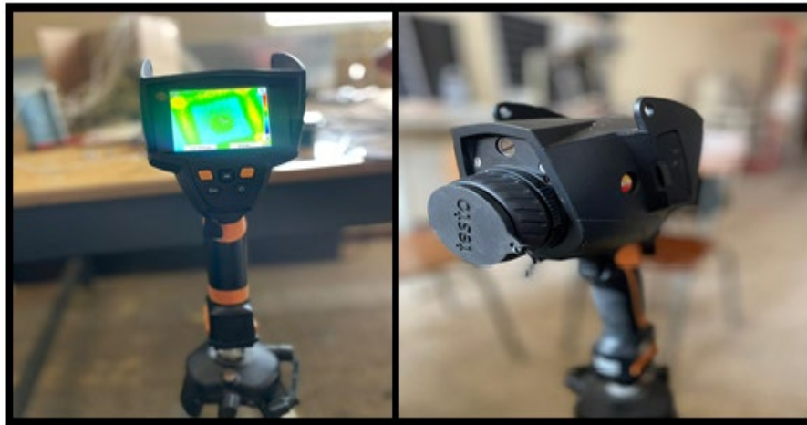
Fig III.11. Camera thermique (IRSoft Testo i875)
