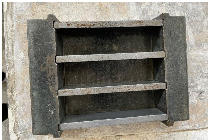
Figure 35: moule ( 4 \times 4 \times 16 \text{ cm}^3 )
