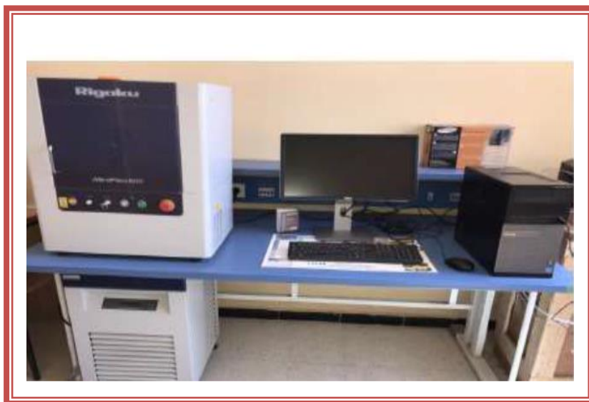
Figure II.8: Appareil DRX -Rigaku Miniflex 600-
