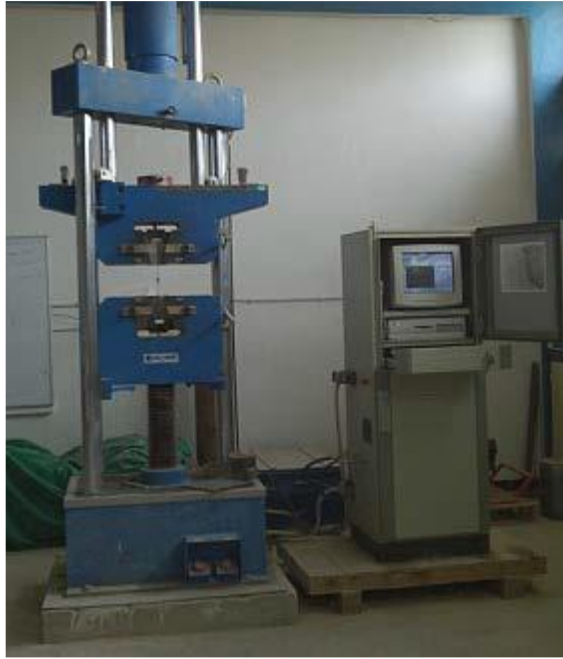
Figure III. 1: Machine de traction Controlab 600 KN
