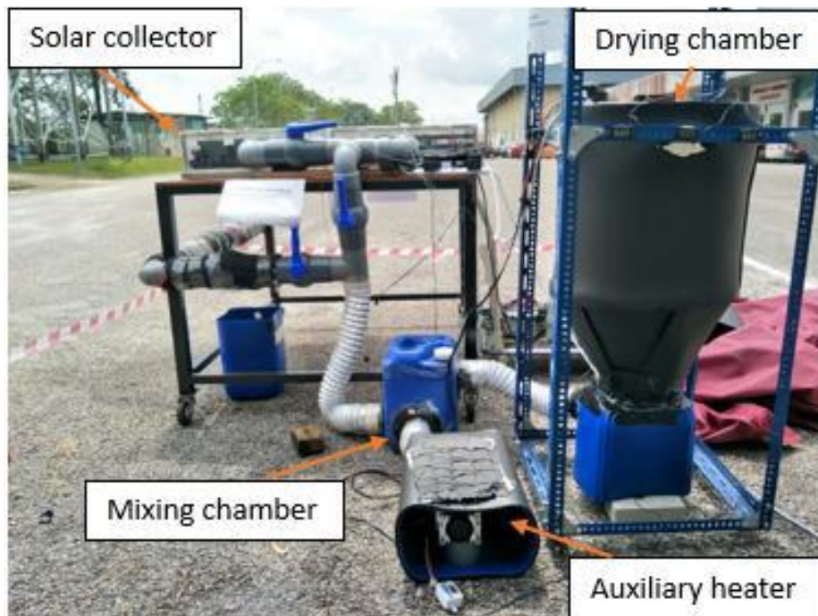
Figure II. 28. Experimental setup of solar drying system swirling drying chamber[68]
