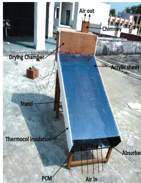
Figure II. 12. Experimental setup of indirect mode solar dryer[55]
