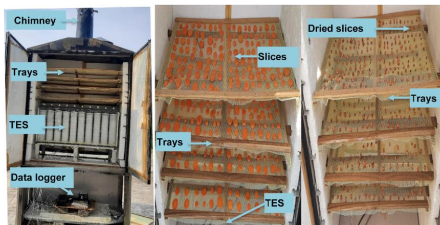
Figure II. 16. Photo snapshot of (a) inside view of setup-II, (b) sliced carrot slices and (c) dried carrot slices[58]
