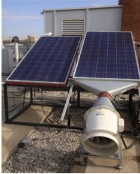
Figure III. 12: Forced Ventilation system [48]
