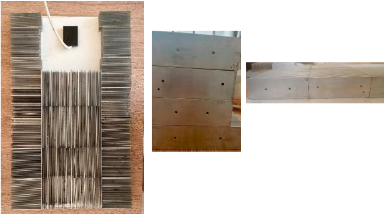
Figure IV. 26: New fins shape (cross fins perforated)
