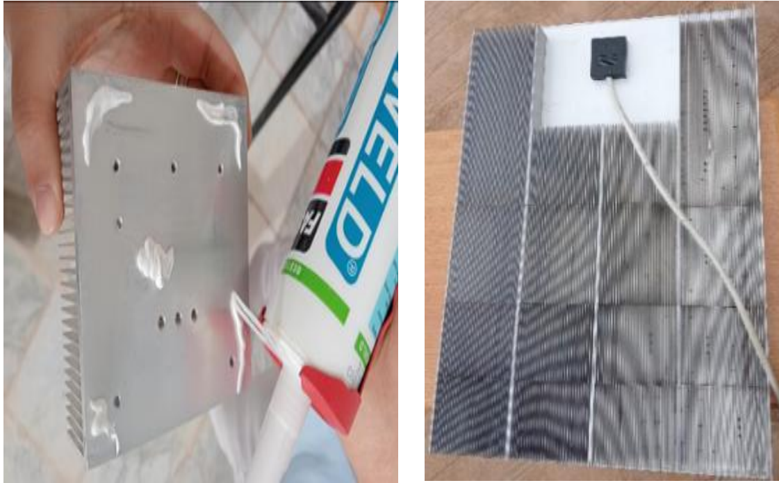
Figure IV. 3: Stick fins on solar panel
