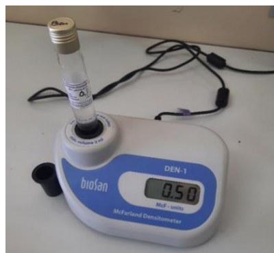
Figure 27: measuring turbidity of inoculum using McFarland Densitometer
