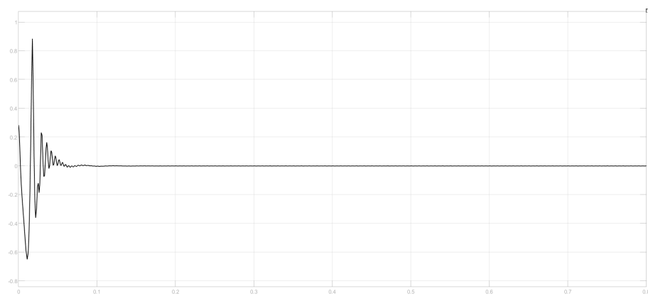
The graph of the Rotor Flux Estimation Error \Delta(\psi_r)
