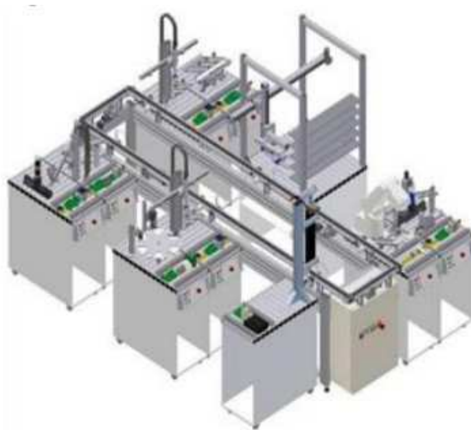
Figure 2.14 : Station MPS 500 de FESTO [9].
