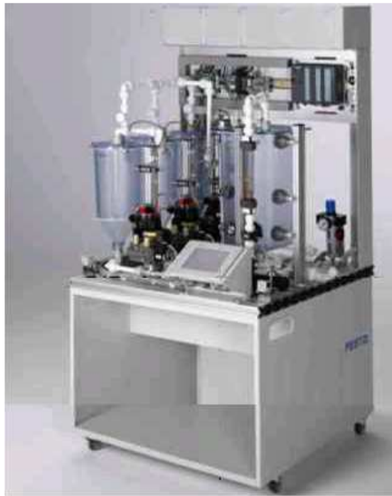
Figure 2.5 : Station de mélange.
