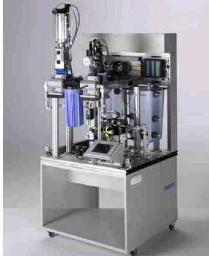
Figure 2.2 : Station de filtration [7].
