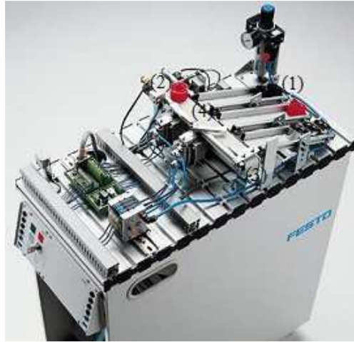
Figure 4.13: Station de tri du MPS 500.
