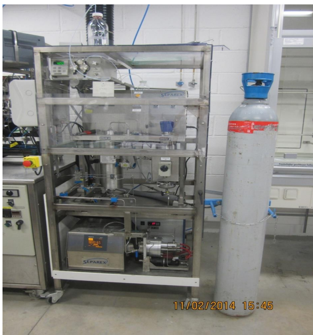
Figure II.5: Installation d'extraction supercritique «SFE1000 bar»
