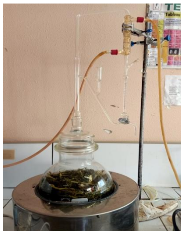
Figure 12. Montage d'hydrodistillation (Clevenger) -photo originale-
