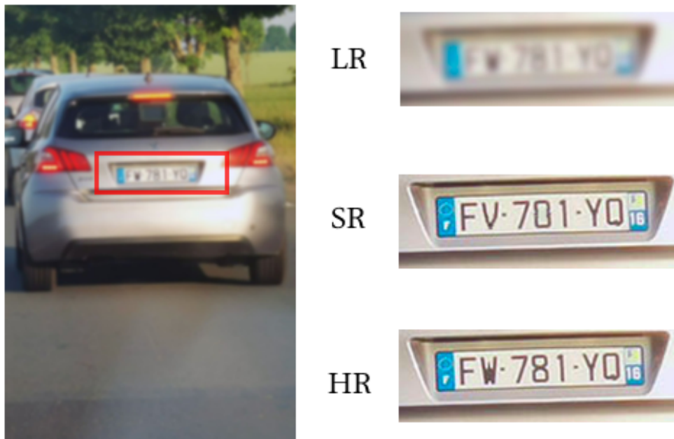
Figure 1.10: Example of a super-resolution (SR) reconstruction error in license plate recognition using SRGAN model, highlighting the need for explainability.
