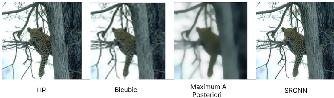
Figure 1.2: Illustration of three categories of image super-resolution: bicubic interpolation (blurry), MAP-based reconstruction (over-smoothed), and learning-based SRCNN (sharper and closer to HR).
