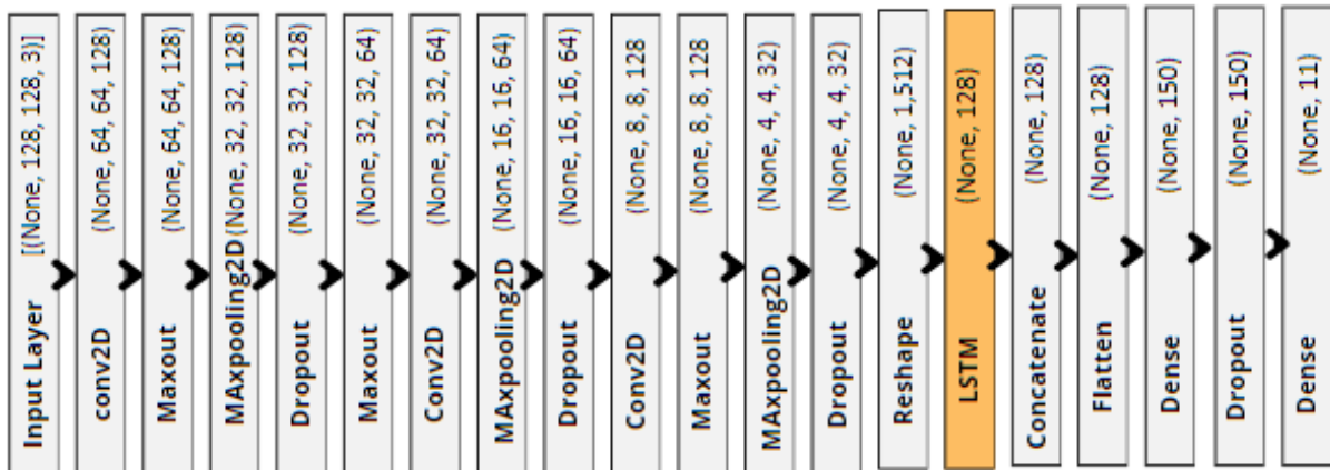
Scheme III- 5: CNN-LSTM used for single input
