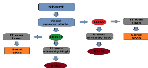
Figure III.10: Flowchart to make loop ()
