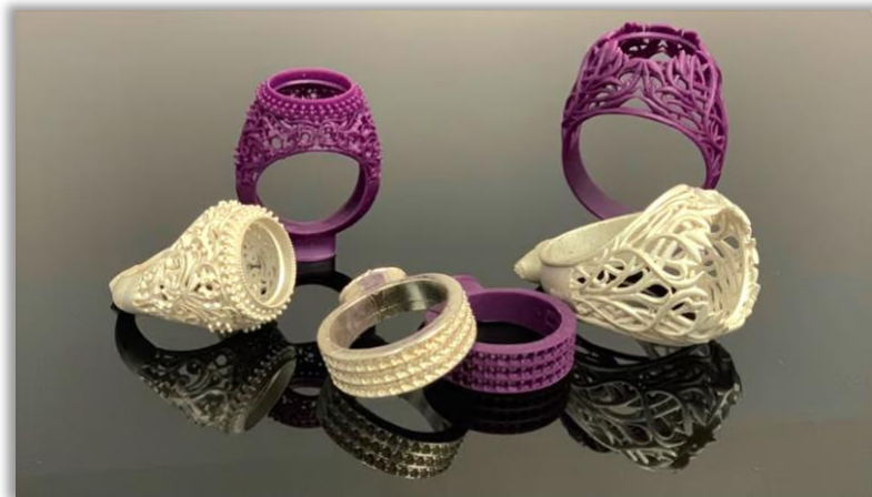
Figure I.4: 3D printed wax jewelry models [6]
