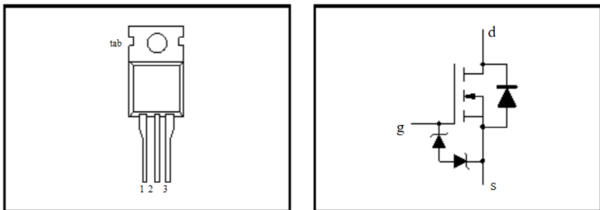
Figure 3.6. IRFZ44N N-Channel 55 V (D-S) MOSFET.[23]
