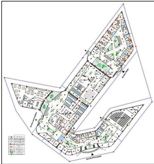
Figure196. Plan protection incendie RDC.
